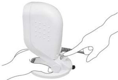
Figure 2: Place cupula in position and hold firmly with one hand.
