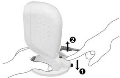
Figure 3: Press down lever to secure device
