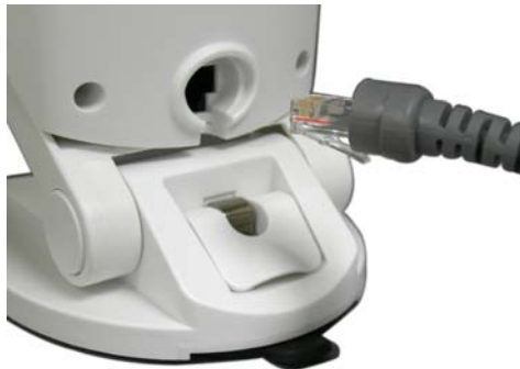
Figure 6: Interface cable connection
