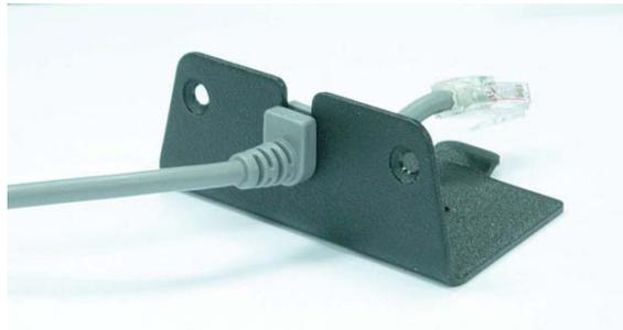
3. Insert the 8-pin modular plug of the power link cable into the “host” connector in the back of the scanner until a firm click is heard.
