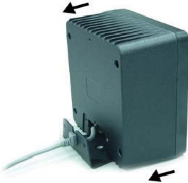
**Install Scanner on Mounting Plate**
